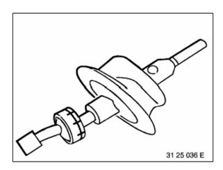
Remove shift lever, refer to 25 11 000 Pull rubber grommet off shift lever.
