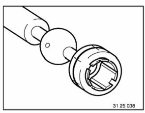
Bearing shell can be taken off shift lever through slots in bearing shell.
